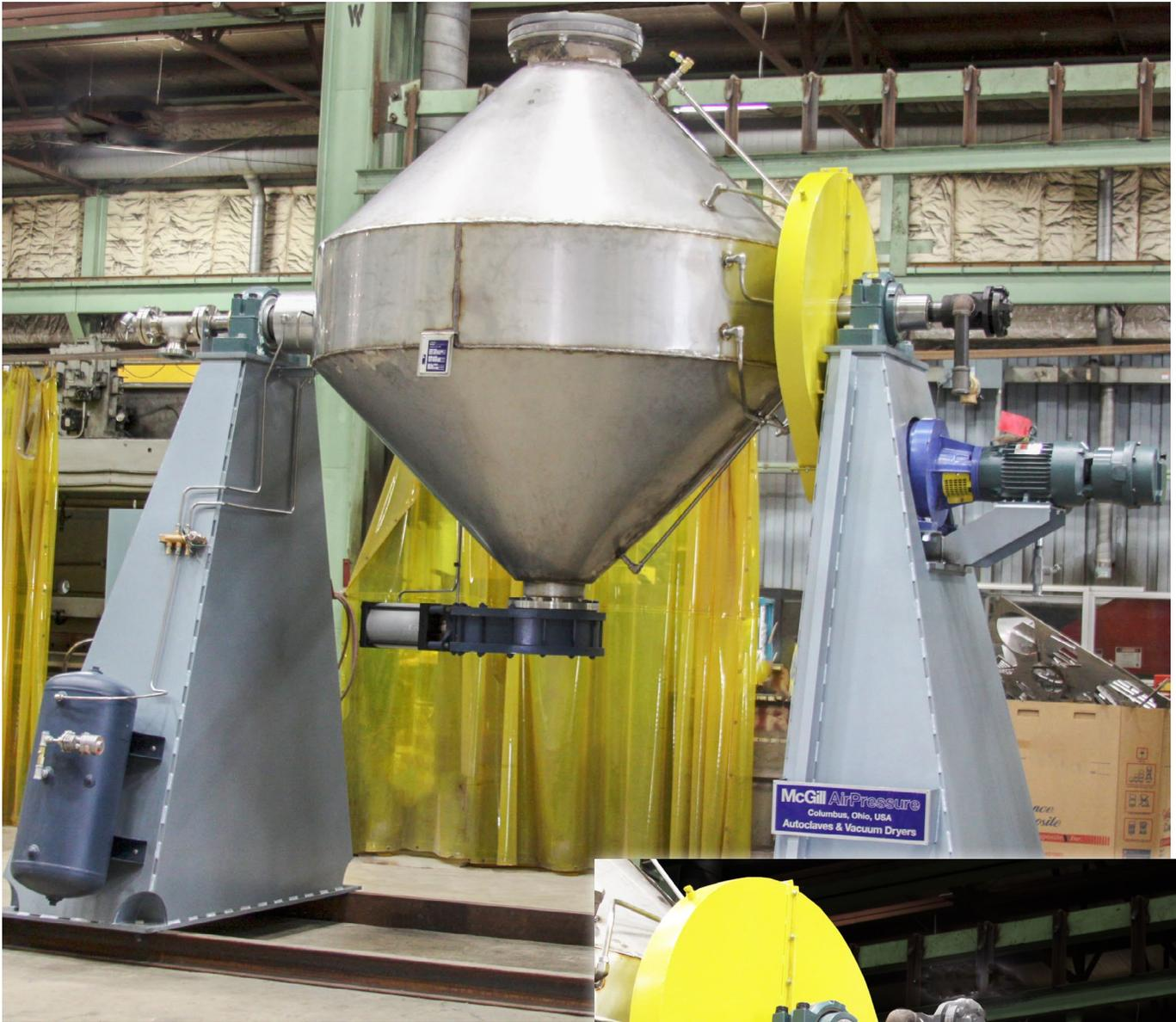
*Above: A vacuum conical dryer designed for processing powdered metals.*
