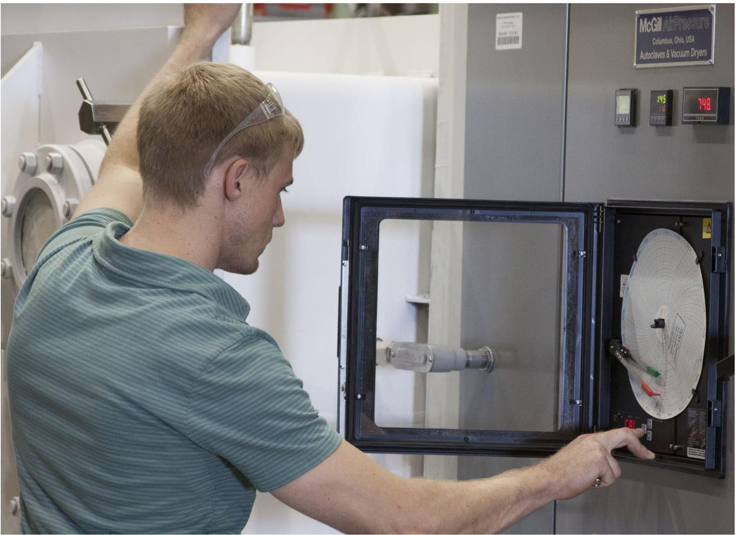
*During testing we can record a variety of test data such as vacuum, temperature, drying time, and moisture reduction level (pictured). From this data we can produce a testing report that provides the information and analysis needed to make accurate and cost-effective recommendations about your vacuum drying equipment requirements.*
