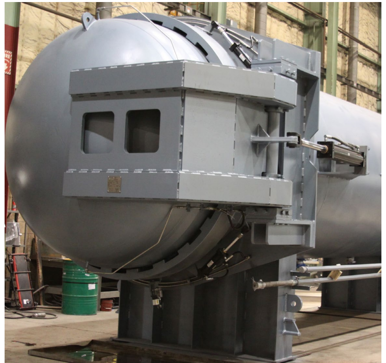
McGill AirPressure's autoclave doors feature rings and lugs machined from solid steel.
