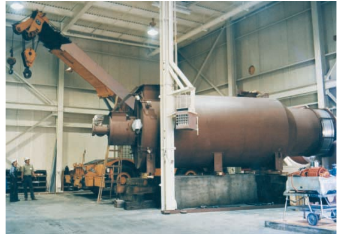
This gas-fired combustion chamber was designed to provide 33 million Btu/hr of heat to a McGill AirPressure autoclave.
