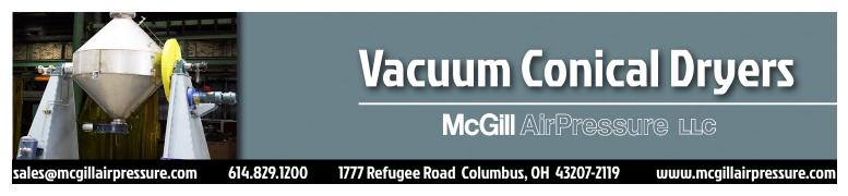
McGill AirPressure designs and manufactures vacuum conical dryers for drying free-flowing materials that cannot stand attrition. Drying takes place in a conical chamber that rotates end over end to create a gentle folding and mixing action. Vacuum dryers remove moisture by exposing the materials to reduced pressure. Just enough heat is used to replace that lost through vaporization.
