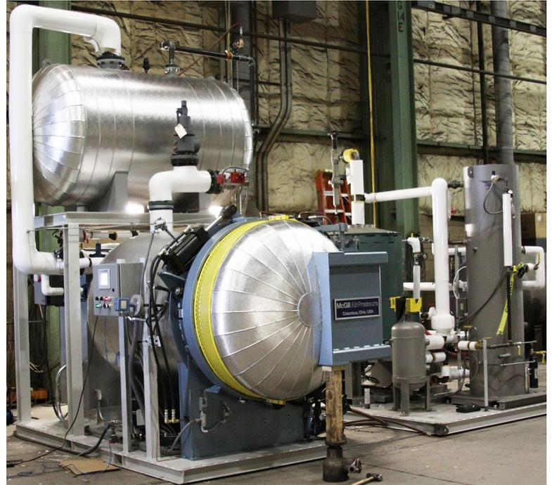
*McGill AirPressure's dewaxing autoclave systems are delivered as a complete, ready-to-install package.*
