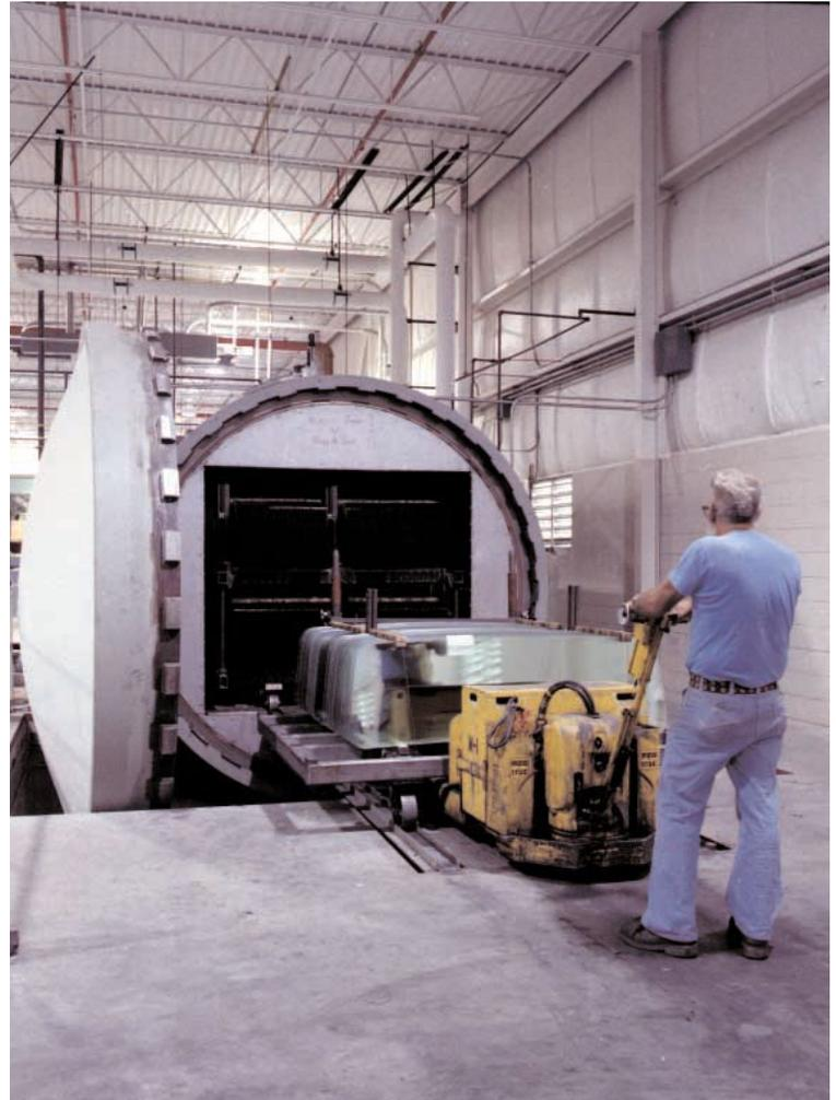
*Mini-Bonder autoclave systems are shipped completely assembled, piped, and wired. The system's internals include insulation, sheet metal shroud, ductwork, blower, blower drive assembly, electrical heater assembly, and cooling coil.*
