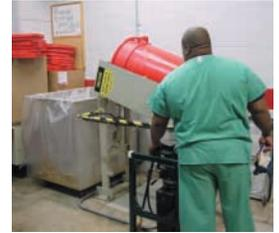
The sterilization process begins as medical waste collection containers are dumped into the sterilization cart.
