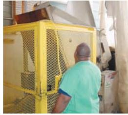
A cart dumper empties the treated waste into the shredder.
