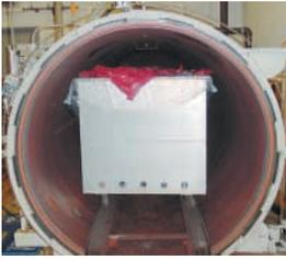
Carts containing bags of medical waste are loaded into the autoclave, a vacuum is drawn, and saturated steam permeates and sterilizes the waste.
