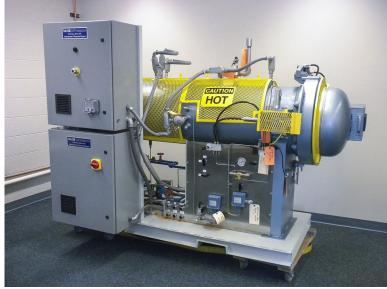
Mini-Bonder autoclave systems are shipped completely assembled, piped, and wired. The system's internals include insulation, sheet metal shroud, ductwork, blower, blower drive assembly, electrical heater assembly, and cooling coil.
