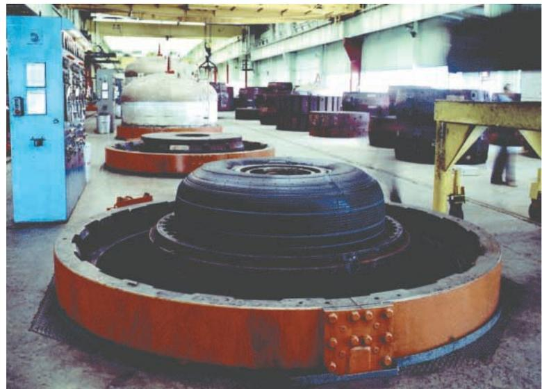
*McGill AirPressure designed and manufactured this series of rubber curing autoclaves for a major supplier of large off-the-road tires.*
