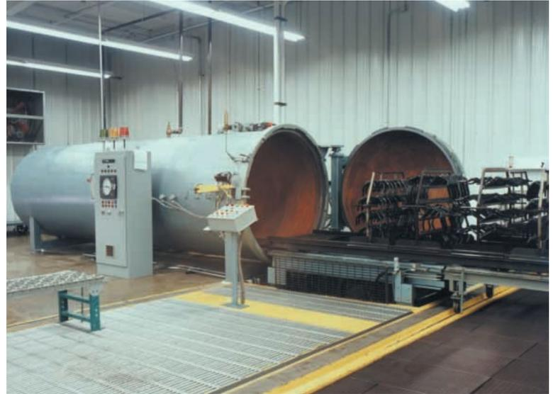
*This McGill AirPressure vulcanizing autoclave system, which included the bridge, load carts, and control system, is used to manufacture specialty rubber hose.*
